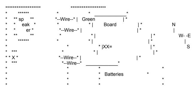
ok...the wire connect the greeen board to the speaker and some silver thing, which I have no idea what the function is. The part you want to modify is the XX=, which represent the crystal. This crystal is somewhat cylndrical shaped, silver, and has two prongs soldered to the board. Unsolder the crystal and replace with the 6.5536 or 6.5000, which is about 2 times as big. You might have to place the new crystal in a somewhat different location, I did the following:
