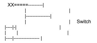
The crystals will share a common ground and have seperate hot wires so that when you switch to one position you have one crystal and the other position will be the other crystal....this SPDT switch can be gotten at Shit Shack (Radio Shack)
